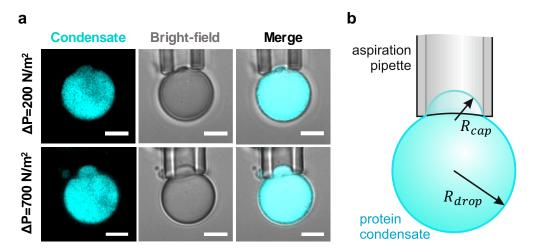
**Supplementary Figure 13.** Micropipette aspiration of a glycinin condensate (cyan) used to assess the condensate interfacial tension  $\Sigma_{ce}$ . (a) Only a small part of the condensate can be aspirated. Beyond certain pressure, the condensate cannot be further aspirated or released. Scale bar: 5 µm. (b) A sketch of the system with the relevant geometrical characteristics used to deduce the interfacial tension (see Methods section on glycinin condensates material properties).
